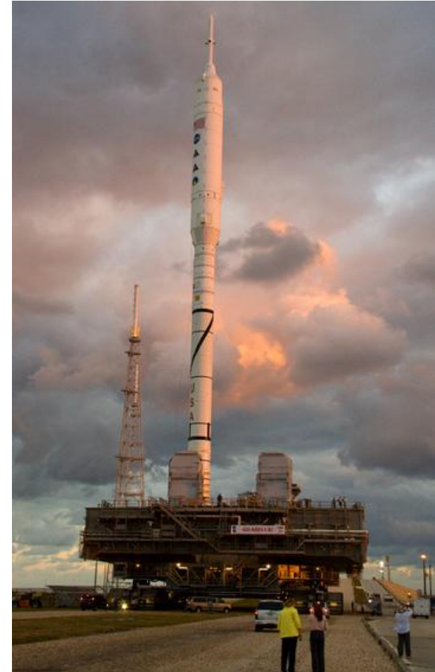
Rollout Configuration: FTV on Mobile Launcher Platform (MLP) and Crawler Transporter(CT)
