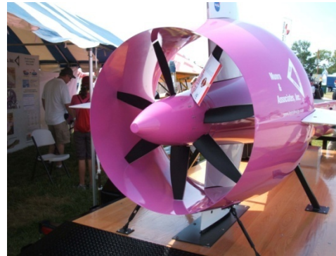
NASA Tailfan Low Noise Duct, 2006
