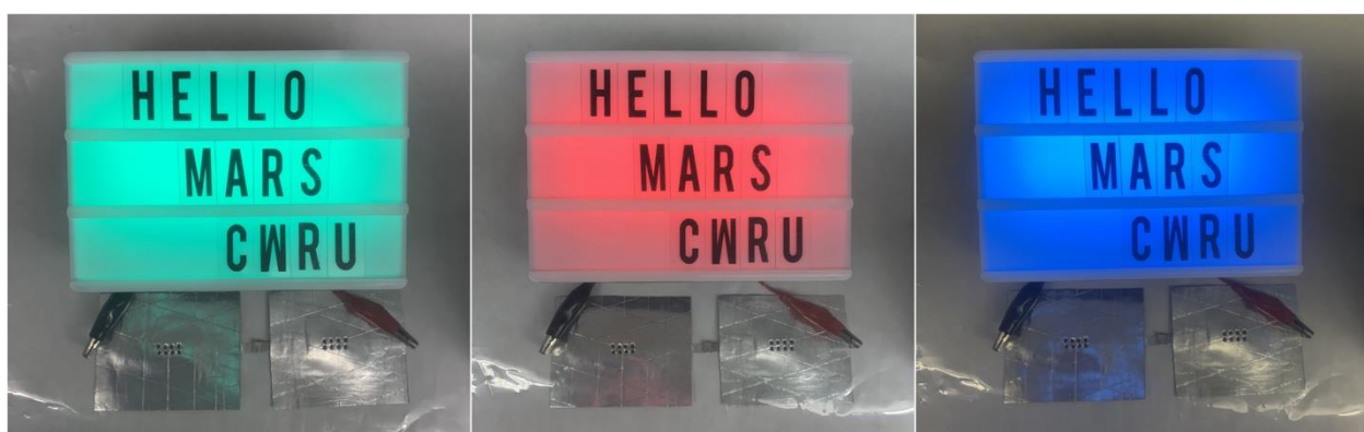
Fig. S17. Digital pictures of two N,S-doped CNTs based quasi-solid-state flexible Li-CO 2 batteries powering a cinema light box with different colors.
