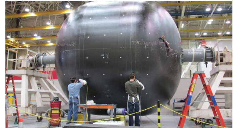
5 m diameter composite LH2 tank (Boeing/NASA)
