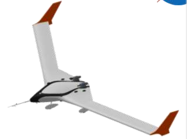
X-56A (MUTT) testbed for flight testing of control laws
