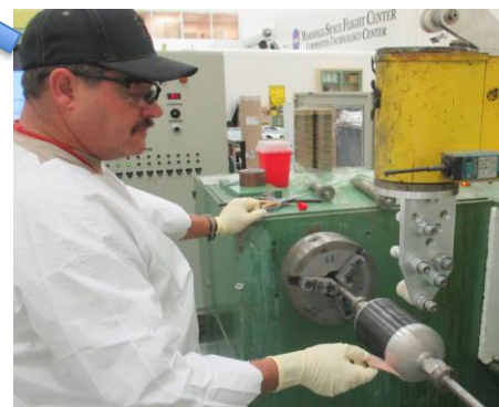
Transfer of CNT processing method to commercial winder at MSFC to manufacture flight test article
