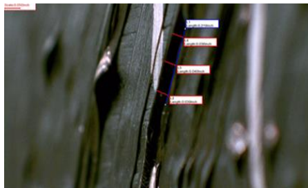
Tape Buckling Defects
