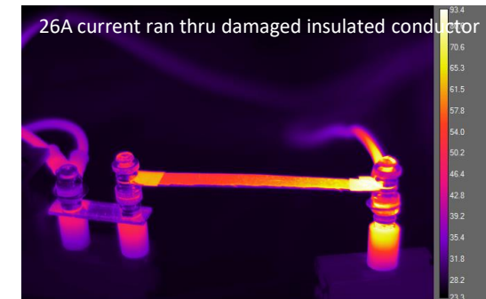
Prototype testing of self-healing insulation
