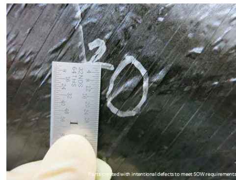
“Pucker” defect formed during steering of 0.25” wide tape on complex-contour part
