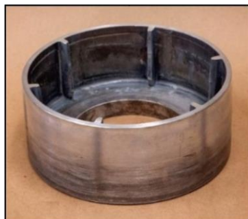
FY12-13 Increased Stiffener Spacing and Height
