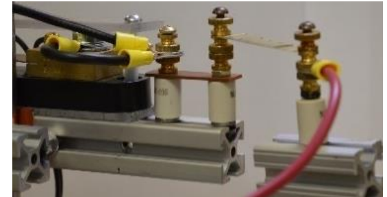
Custom test apparatus to assess real-time scratch healing under simulated use conditions.
