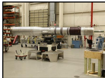
Transfer of CNT processing method to commercial winder at MSFC to manufacture flight test article
