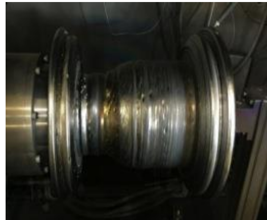
Structural Inconel 625 jacket EBF 3 deposited onto SLM Cu liner
