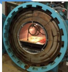
Curing (Autoclave, ovens, thermal presses)
