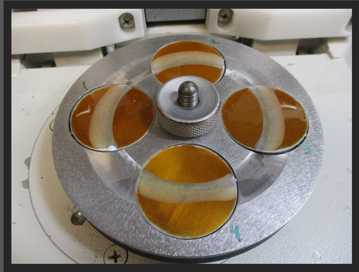
Epoxy APB 1,3,4 - D.E.R. 331 - P.E.G.: 35% - Coated 7/8/2019 Taber Abrasion Tested on: 7/12/2019
