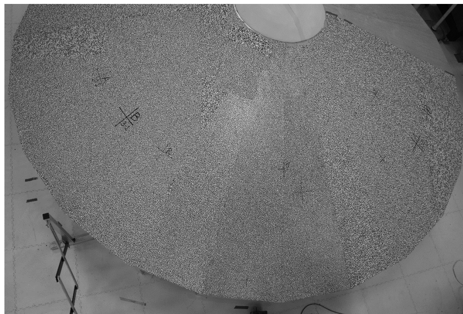
3D DIC camera view of surface of Mock-up Heat Shield
