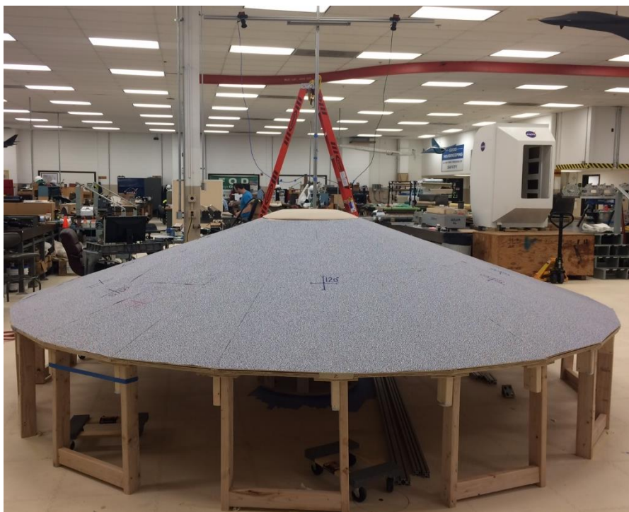
Mock-up Heat Shield with printed speckle pattern applied (printed on paper)
