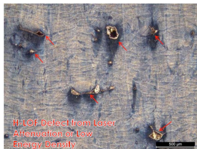
Defects due to inadequate ventilation on the powder bed.
