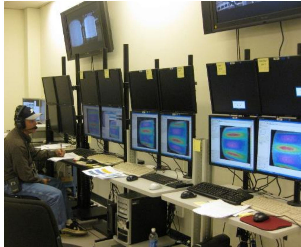
Control Room with VIC-3D™ Real-time Monitoring of each system
