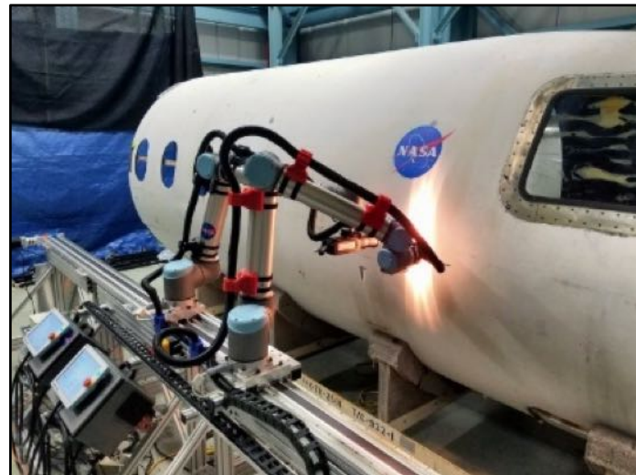
Dual Collaborative Robot Line Scan Thermography
