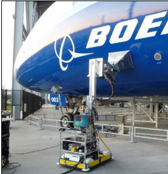
Automated UT Enhancement to IR Inspection (GIRAFFE)
