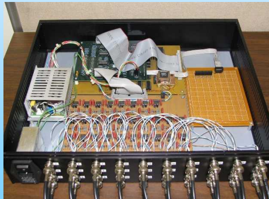
State Estimation Fusion Processor For Flow Control (Humphreys, 2008)
