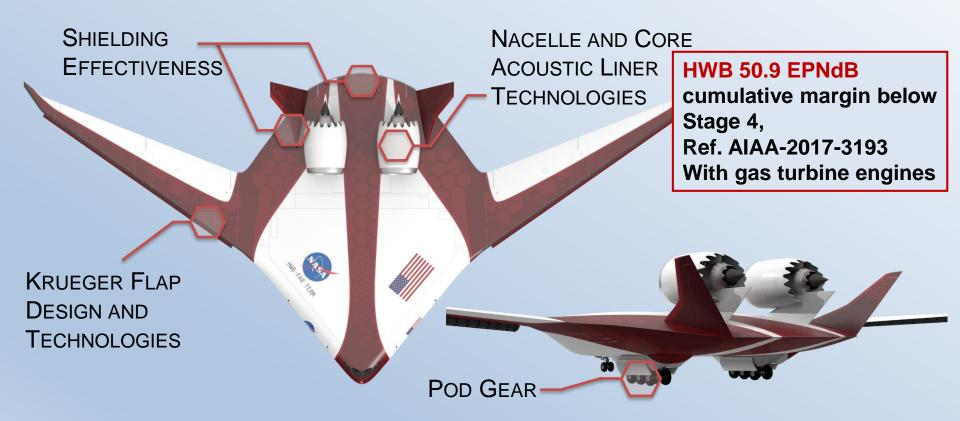
Low noise possible through configuration change, Electrification could enable low noise *IF* designed for noise from beginning
