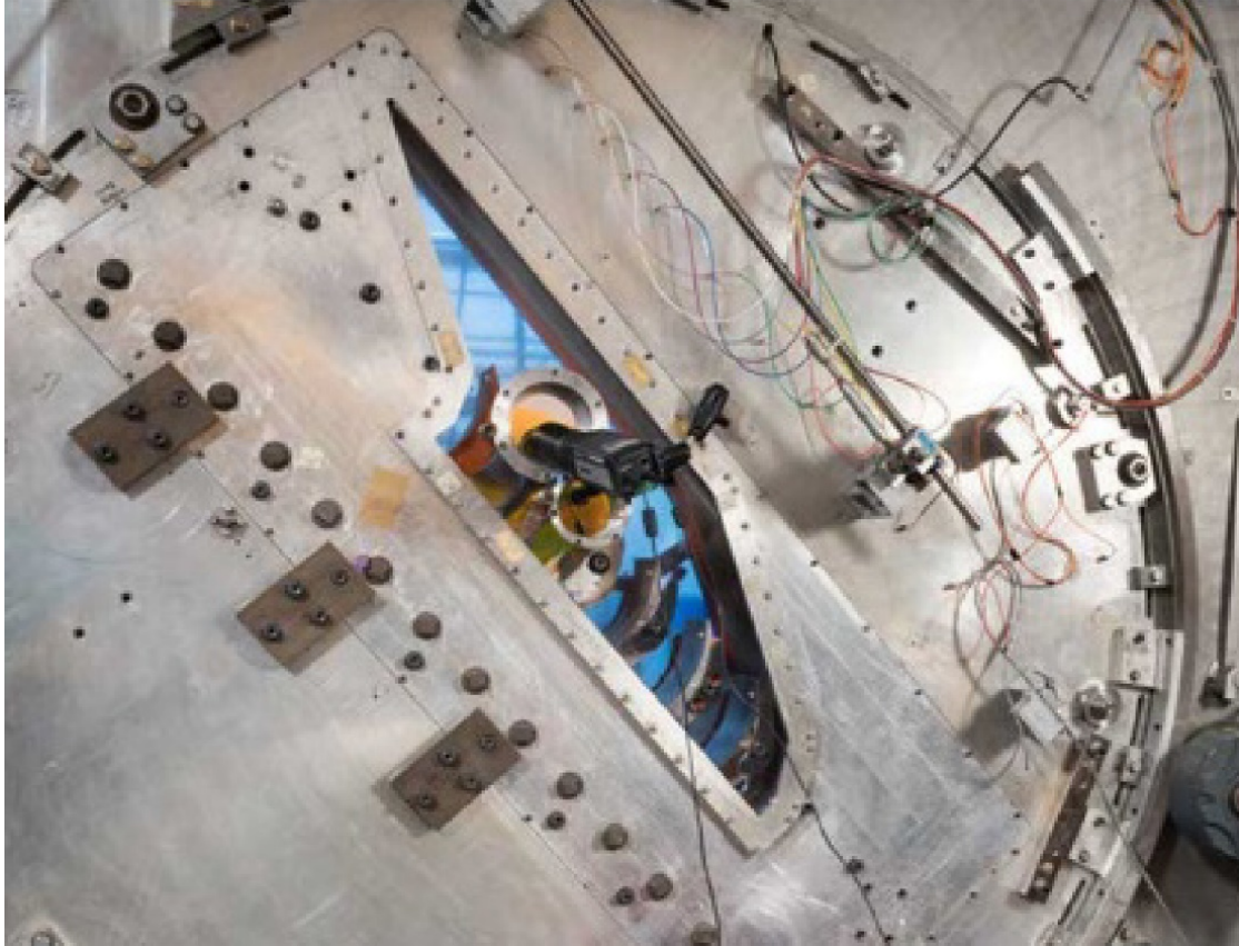
Figure 4.—Infrared window ports and cameras in Transonic Turbine Blade Cascade Test Facility.
