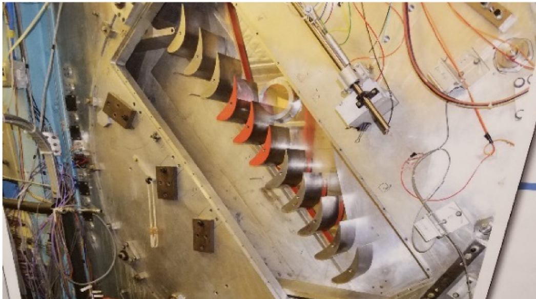
Figure 1.—Transonic Turbine Blade Cascade Test Facility. (a) Cascade wheel. (b) Test section.
