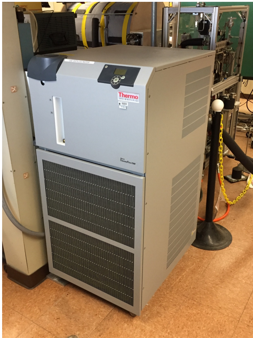
Figure 22.—Thermo Scientific NESLAB ThermoFlex™ 7500 recirculating chiller.
