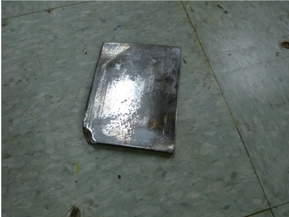
Figure D.22.—LG1115 posttest projectile.
