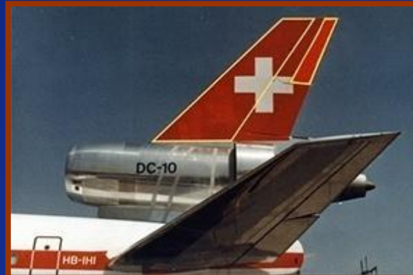
Douglas DC-10 composite Rudder and vertical stabilizer
