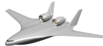
N2A - Poded engine model to be tested
