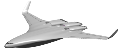
N2B - Embedded engine model studied
