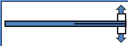
Double Cantilever Beam (DCB)
