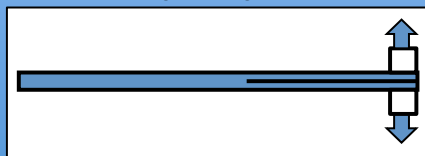
Double Cantilever Beam (DCB)
