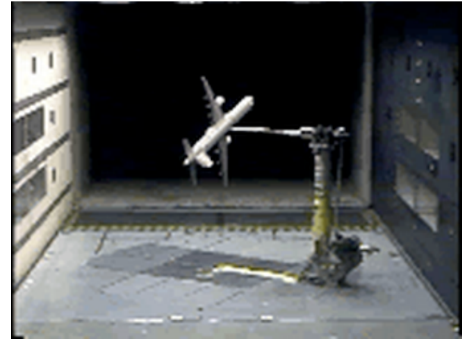
5.5% model on yaw forced oscillation rig NASA LaRC 14x22 Ft Tunnel
