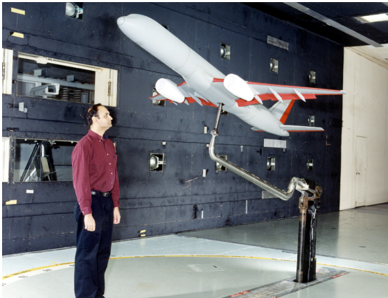
5.5% model on static mount NASA LaRC 14x22 Ft Tunnel
