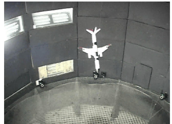
2% free-spin model NASA LaRC 20-ft Vertical Spin Tunnel
