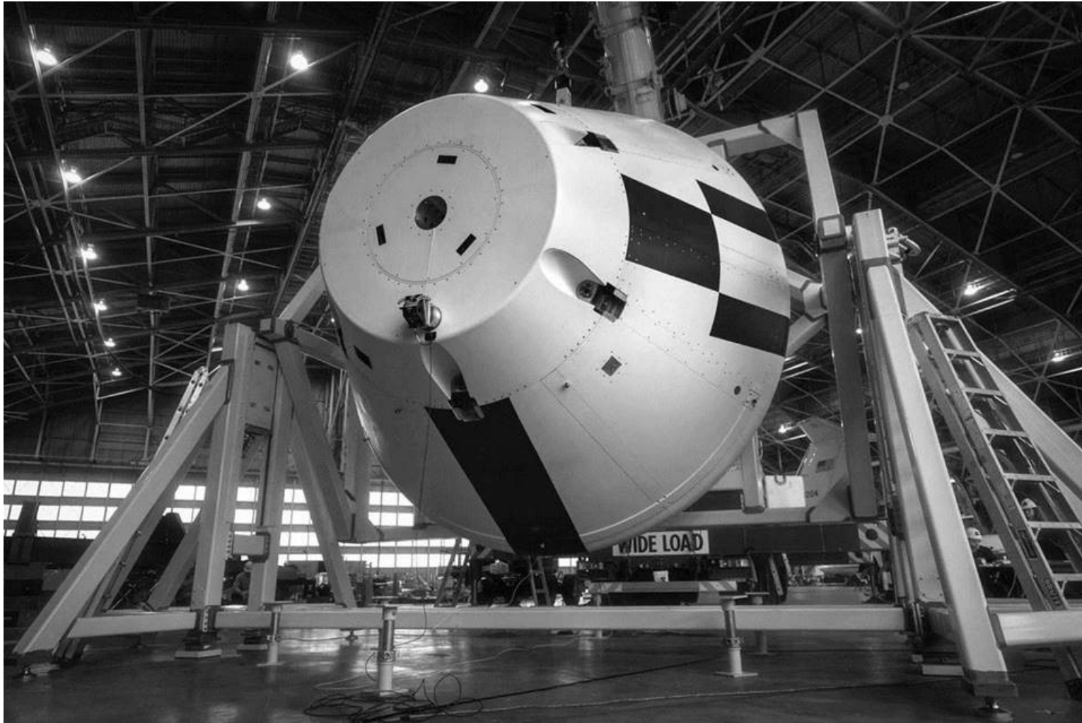
AA-2 CM Boilerplate X-CG measurement at LaRC with structure and ballast installed. Measurements successfully taken while using mobile crane.
