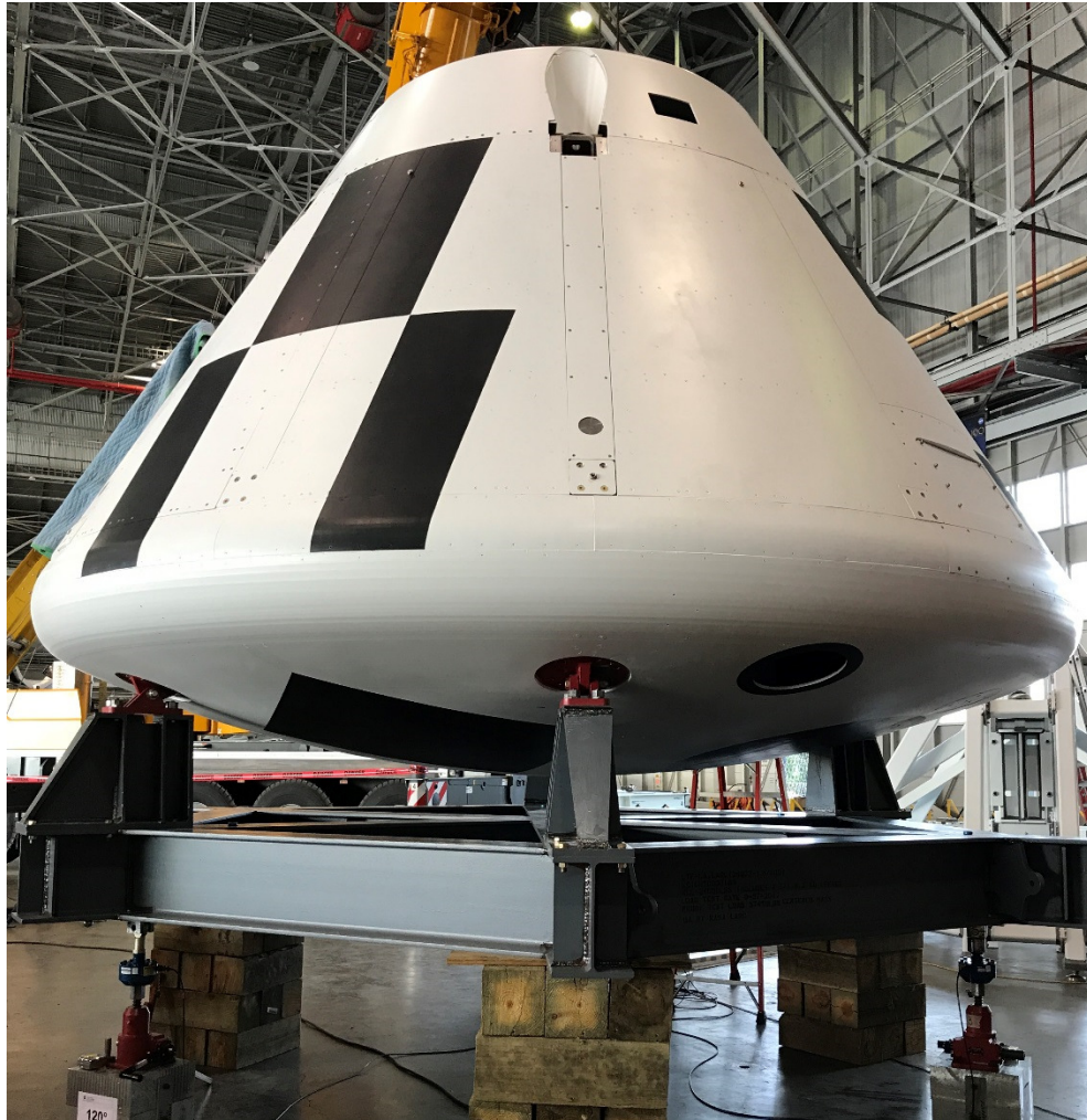
AA-2 CM Boilerplate Y and Z CG measurement at LaRC with structure and ballast installed prior to shipment to JSC. Measurements successfully taken while using mobile crane.
