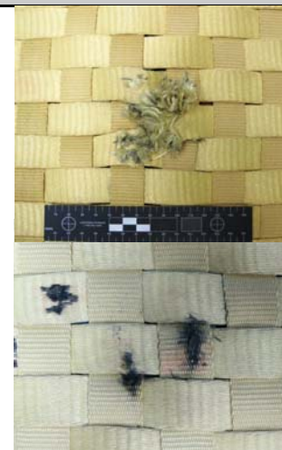
Hypervelocity Impact on Protected Restraint (TransHab)
