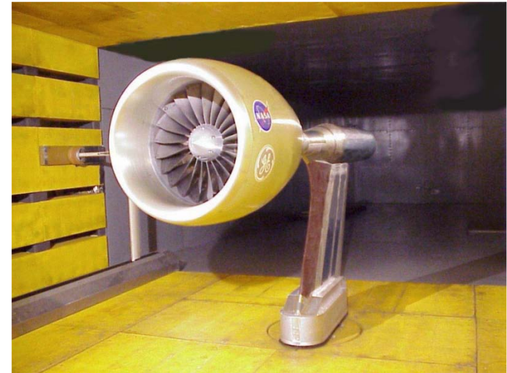
Scale Model Test 22" Fan Rig in GRC 9'x15' Wind Tunnel
