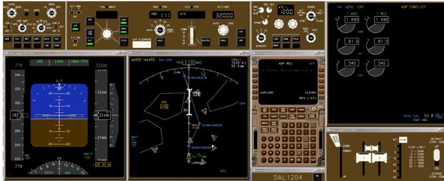
Aircraft Simulation for Traffic Operations Research (ASTOR) Pilot Interface
