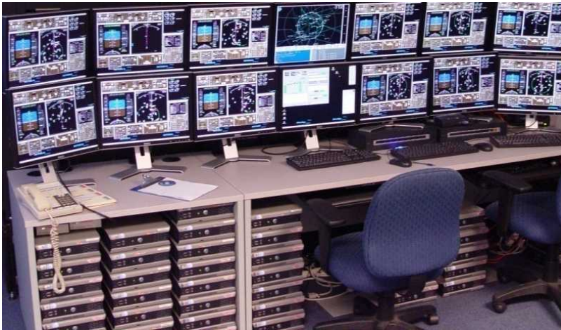
Over 500 aircraft can be simulated – each aircraft is simulated on a single computer
