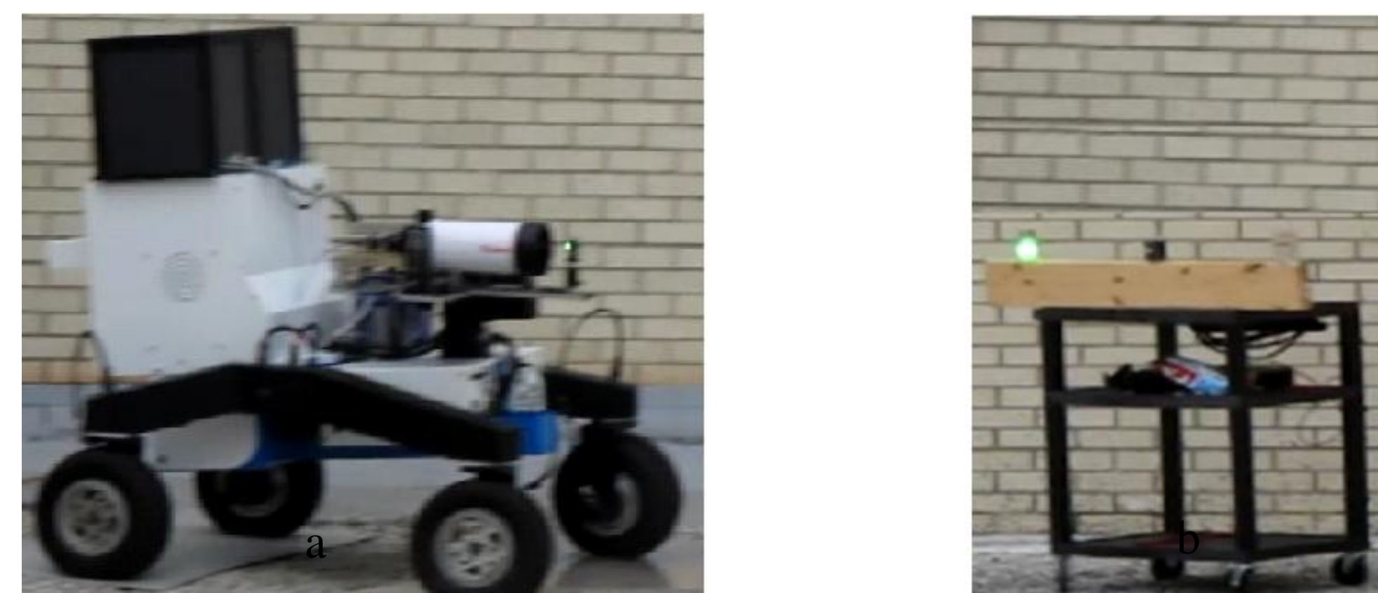
Laser beam in (a) pointed to the surface target sample in (b) at a 15 meter distance
