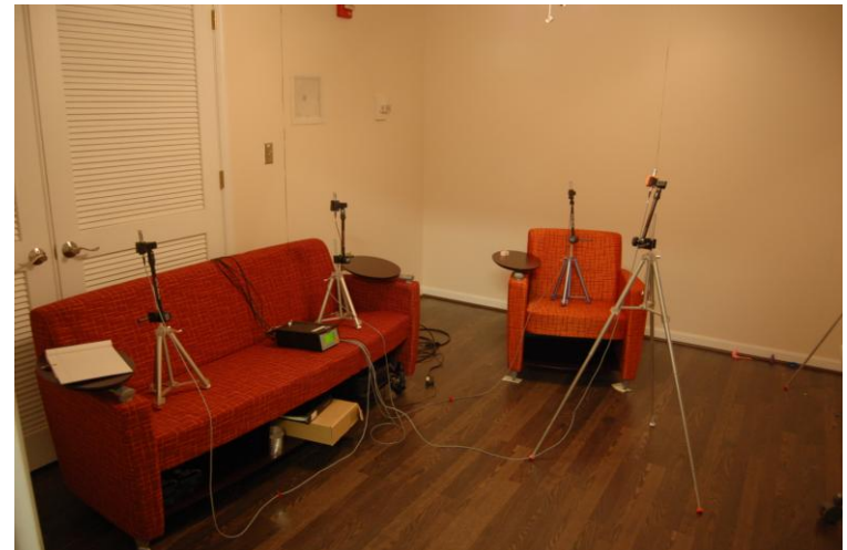
Microphone locations inside IER
