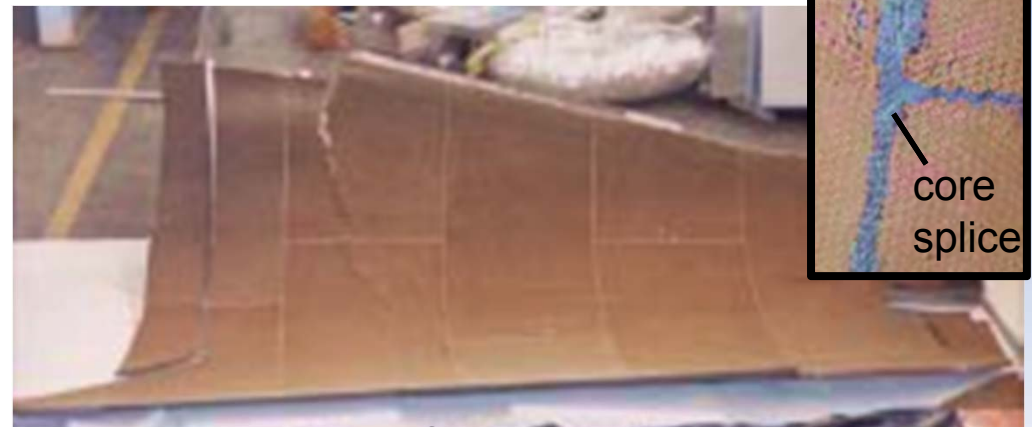
Removed outer facesheet and core (showing core splices)
