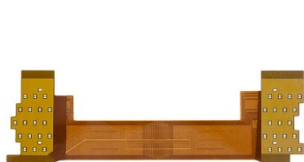
Basic Meandering Winding Magnetometer (MWM) design
