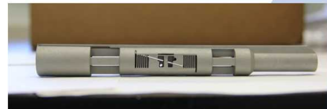
0.75 inch dia. Balance produced from 17-4 using ADM
