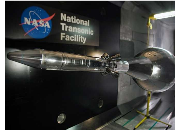
Launch Abort System model in the National Transonic Facility
