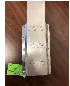
THX Phase 4 plate concept (3 arrays of cooling holes).
