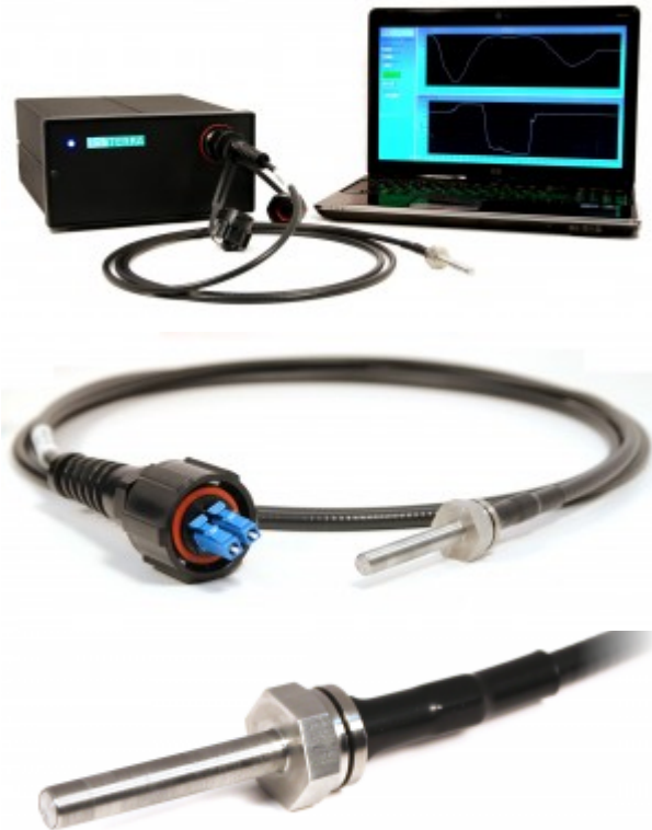
Commercially available shear stress measurement system
