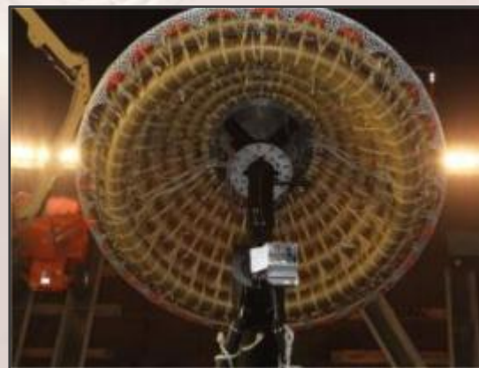
Photographs of inflatable structure and flexible TPS
