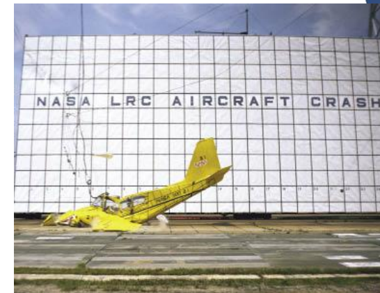
Full-scale GA Airplane Crash Testing at LandIR from 1970's
