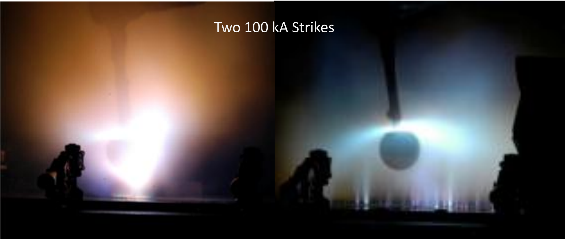
4 second time lapse photograph showing Lightning Strike Attachment on Mesh Protected CFRP Panel
