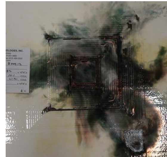
Post Strike Damage 27
