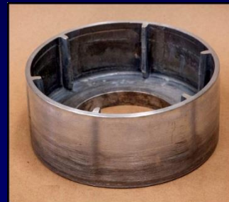
First Attempt at Forming Cryogenic Tank Stiffener Shape
