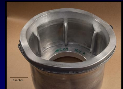
Forming with Multiple Stiffener Shapes
