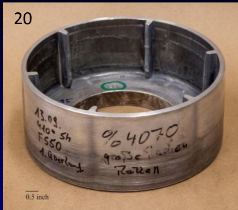
Best formed cylinder; single pass (Parameters used in 2014 experiments)
