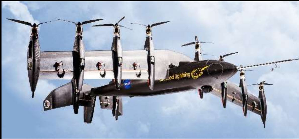
GL-10 sUAS DEP Tilt-Wing Tilt-Tail Vertical Takeoff and Landing (VTOL) Demonstrator (Fully Redundant Vehicle Thrust Solution)
