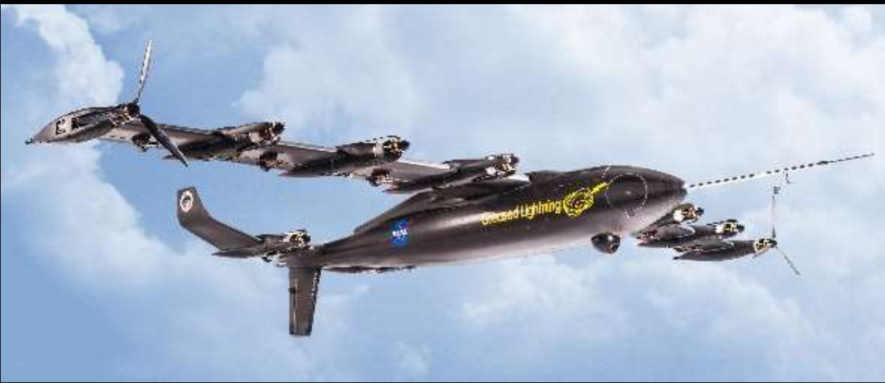
GL-10 sUAS DEP Tilt-Wing Tilt-Tail Vertical Takeoff and Landing (VTOL) Demonstrator (Fully Redundant Vehicle Thrust Solution)
