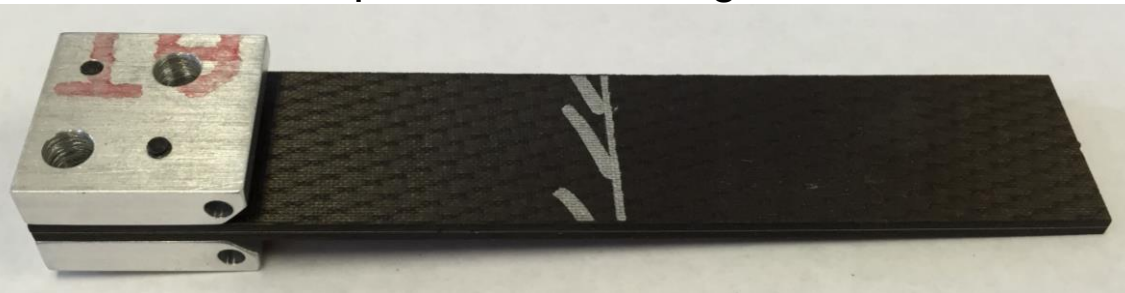
DCB specimen with hinges attached
