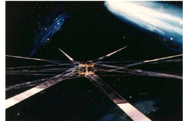
A 15 km diameter heliogyro solar sail was the preferred concept for a proposed JPL Comet Halley rendezvous mission in 1977.
