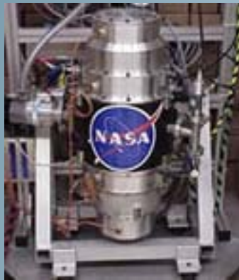
Fly-wheel Power Storage
