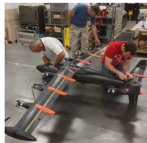
NASA GL-10 sub-scale flight demonstrator (10' span, 62 lbm)
