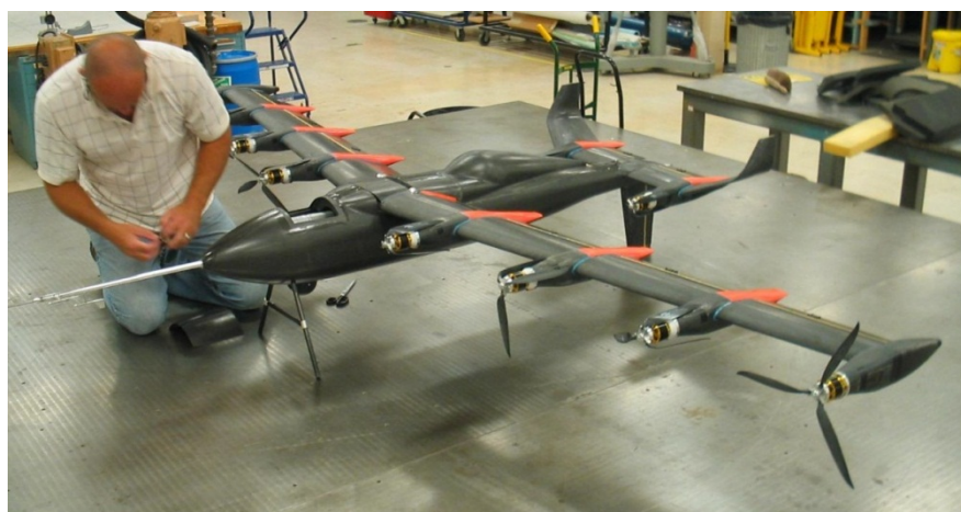
NASA GL-10 sub-scale flight demonstrator (10' span, 62 lbm)
