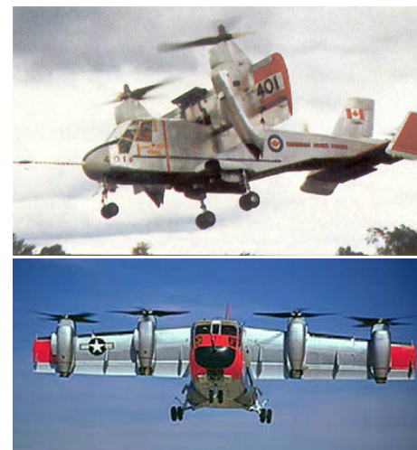
Compare to XC-142 and CL-84 Tiltwings which experienced transition buffet control issues
