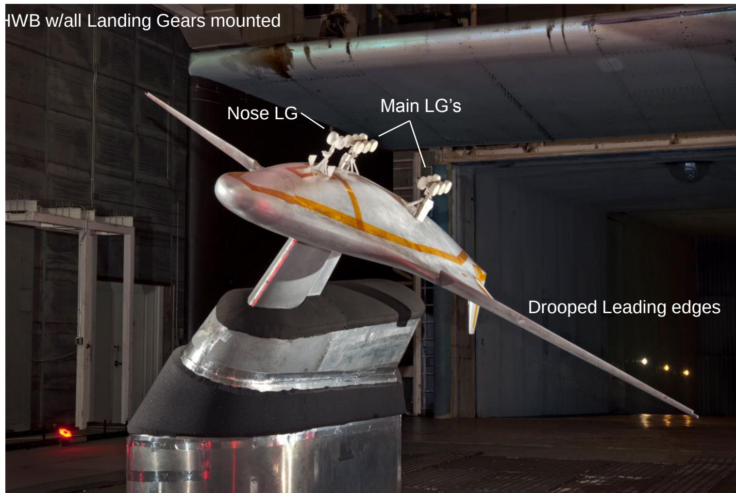
HWB model in 14'x22'test section with 30° roll and configured for airframe noise testing
