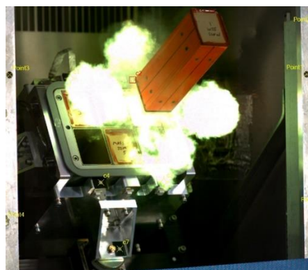
Figure 8: Ejection testing of a data recorder mass simulator.
