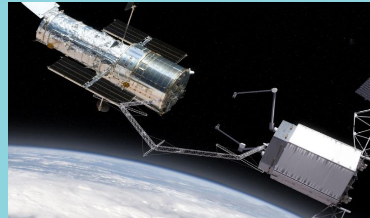
Figure 1: Graphic of ongoing Technology development TALISMAN shown in proposed Satellite Servicing Mission (SSM) (Image Credit: NASA)
