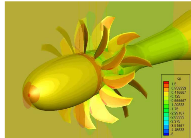
Predicted Cp contours (Isolated)
