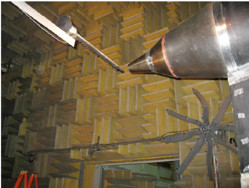
Figure 4. Point noise source mounted 2 inches downstream of the CV Nozzle, Conf. 30000
