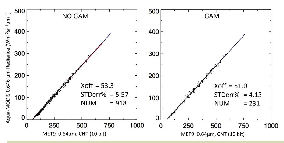
• The X offset or the linear regressed offset is closer to the true space count of 51 using the GAM method
