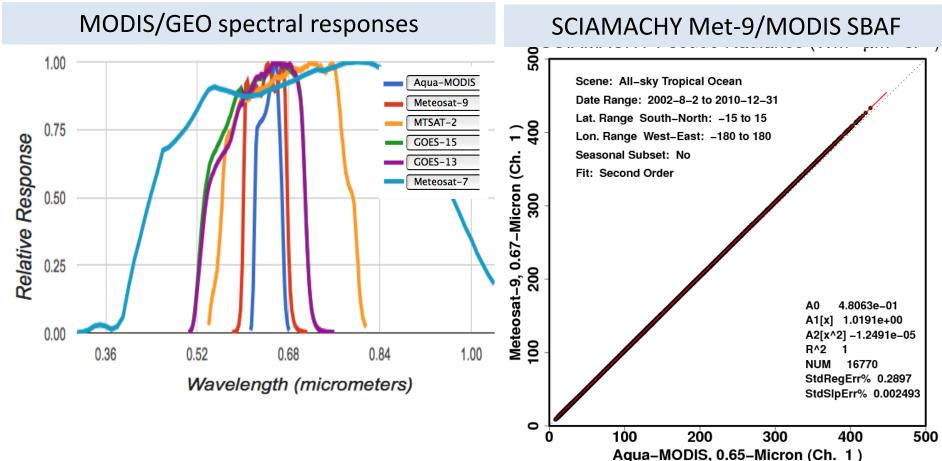
• Convolve the footprint SCIAMACHY hyper-spectral radiances with the Met-9 and MODIS spectral response functions. Regress the SCIAMACHY pseudo radiances over the raymatching domain. Apply the SCIAMACHY SBAF to the MODIS radiances.
