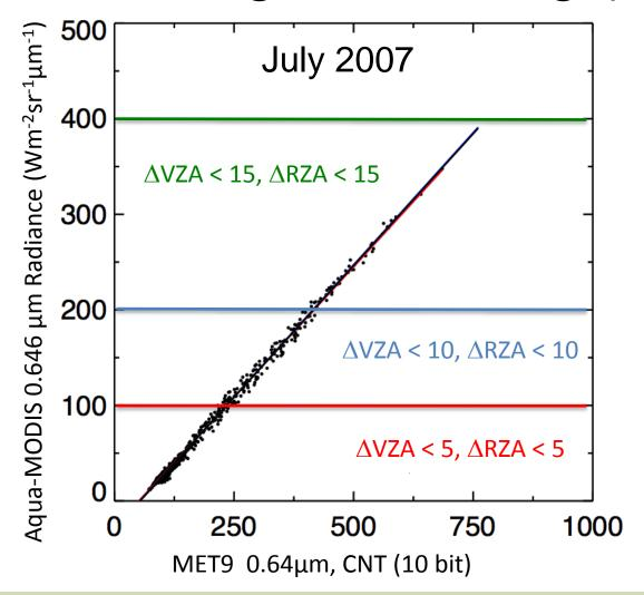
• Split the Aqua-radiance domain into 3 sections, increase the angular restriction in the lowest 2 sections
