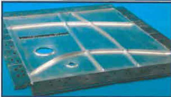
Structurally optimized panel designs & machined test panel
