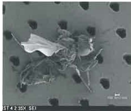
Impacted insect adhesion & blockage of HLFC surface
