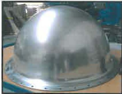
As-formed, no machining 0.6m dia.
