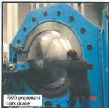
As-formed, no machining ~2m dia.
